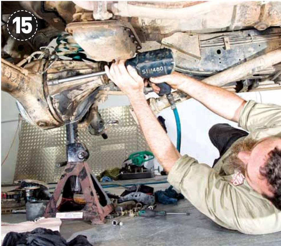
**13** To ensure we're still on track for a quiet diff, check the crownwheel to pinion backlash as the carrier bearing cap bolts are tightened. Once these bolts are tight the backlash should be the same as before we disassembled the diff if all goes to plan
